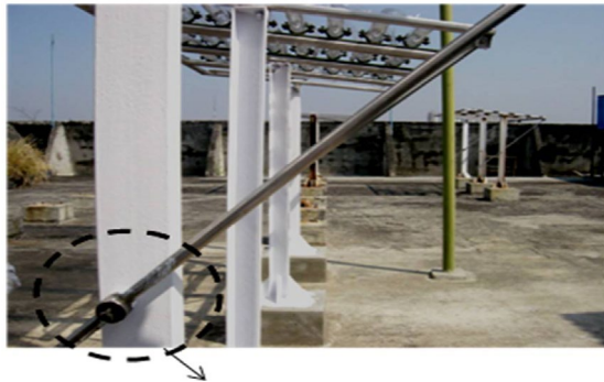
Figure 2. The slope regulator of PBR panel (screw type).
