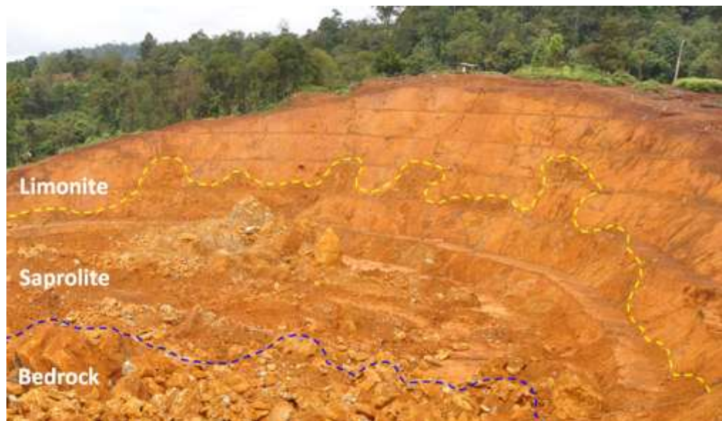
Fig. 4. Laterite profile of unserpentinized ultramafic rock on Sorowako mining face.
