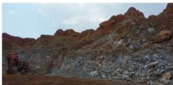
Fig. 8. Example of medium fractured type based on drilled core data
