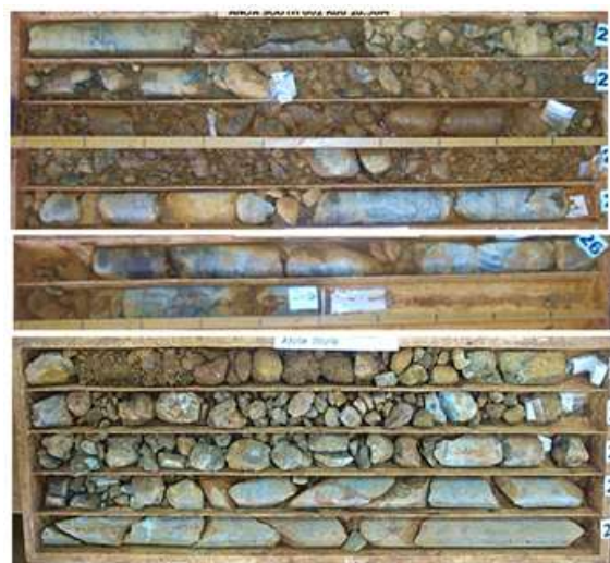
Fig. 8. Example of medium fractured type based on drilled core data
