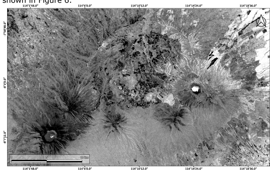
Figure 6. Principal Components from Landsat 8 data for hydroxyl carrier minerals (PC4) are shown as bright pixels.
