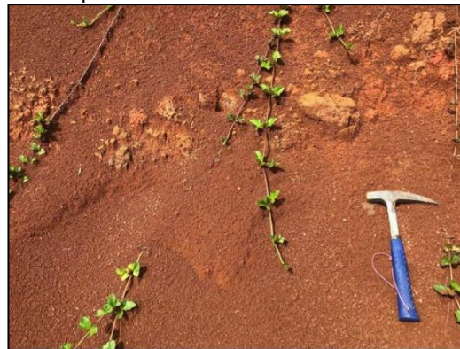
Figure 7. Close-up of the research slope area indicates weathered tuff
