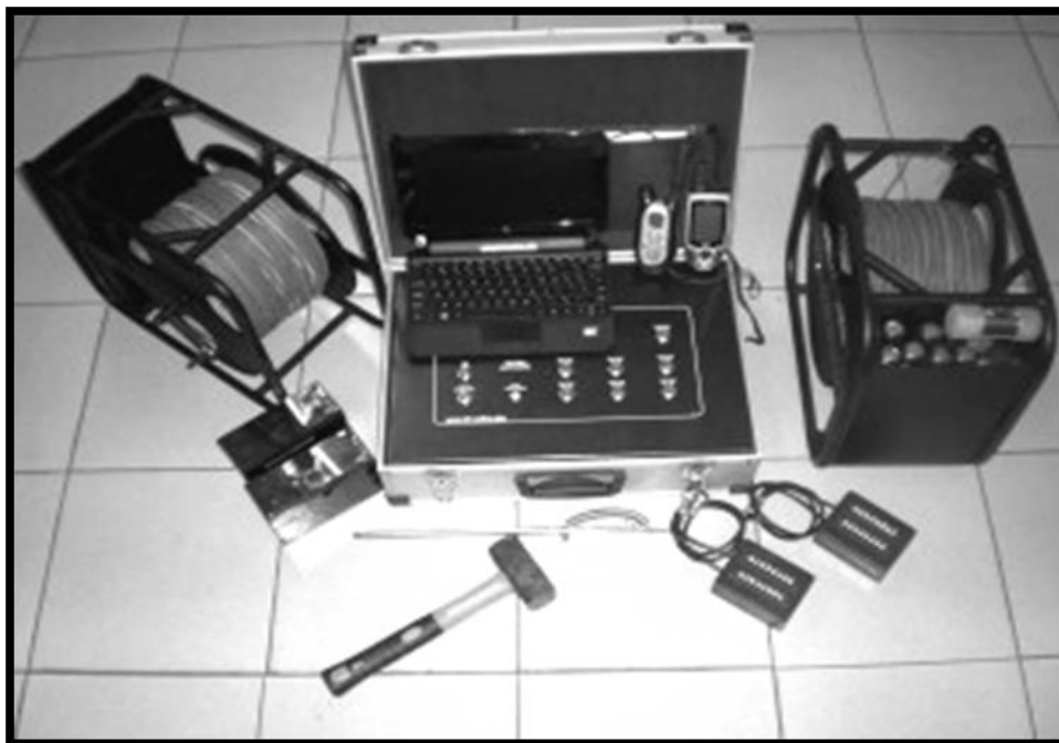
Gambar 2. Alat Resistivitymeter Automatic Multichannel.
