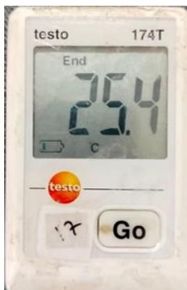
**Gambar 1.** Thermometer Data Logger Testo 174-T
