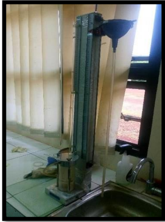
Gambar 3.1 Alat permeameter metode falling head.
