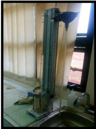
**Gambar 3.1** Alat permeameter metode falling head.
