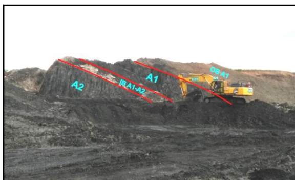
Gambar 2. Kenampakan Overburden A1, seam A1, Interburden A1-A2, dan seam A2.
