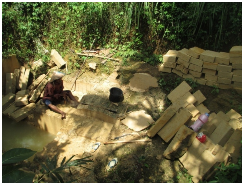
Figure 6 Brick cutting process by sawing.
