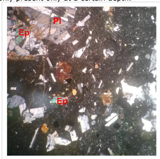
Figure 8. Microscopic photo (magnification 40) at a depth of 330 m, The epidote (Ep) replaced some of plagioclase (Pl).
