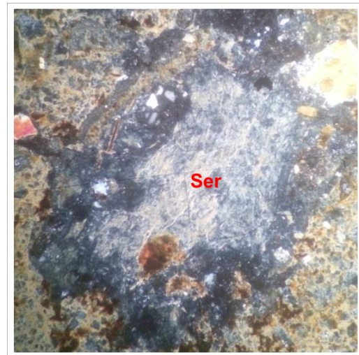
Figure 2. Microscopic photo (magnification 40) at a depth 41.5 m, the sericite (Ser) replaced plagioclase almost entirely.
