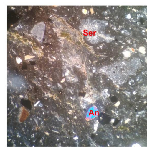
Figure 5. Microscopic photo (magnification 40) at a depth 328 m, anhydrite (An) and sericite (Ser) were present.
