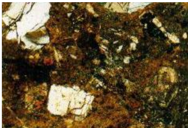
Figure 7. Petrographic section sandstone matrix at breccia outcrops.
