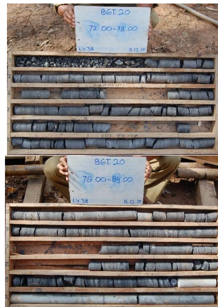
Figure 2. Sample cores drilled for the interburden layer B2 – C.
