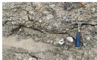
Figure 2 Cracks around the SMD block OPD waste dump area
