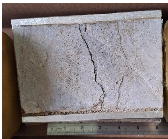
Figure 4. Core Photographs of Bioclastic Wackestone (1572 m).
