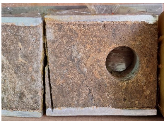
Figure 5. Core Photographs of Bioclastic Packstone (1571 m).
