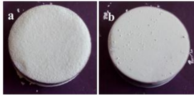
Figure 8. Ti-6Al-4V metal alloy after sheathing (a) nanotubes and (b) non nanotubes
