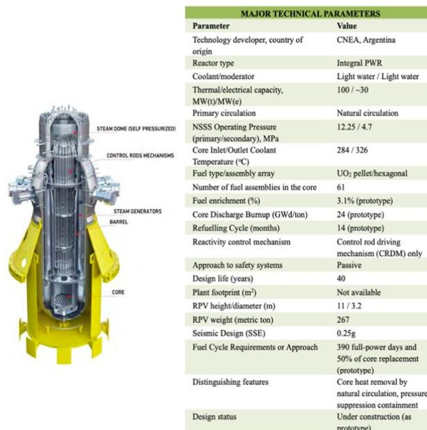
Gambar 3. CAREM Small Modular Reactor System Design
