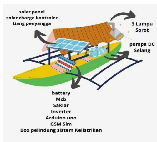
Figure 2. Installation Scheme (Source: Kisat Saksi Editor, 2024)
