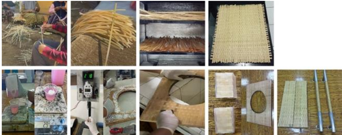
Fig. 4. Route of the Fabrication Process of Bamboo/Glass Fiber/Polyester-Eggshell Powder for the Commode Chair Components.
