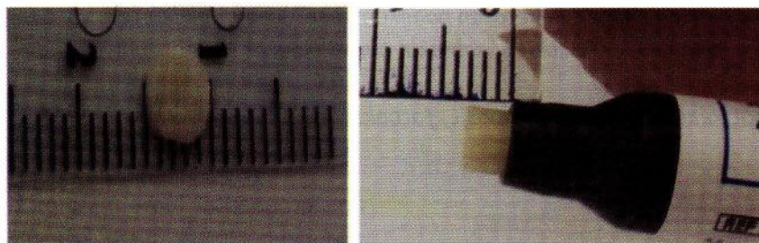
Figure 1. A. composite diameter measurement; B. composite length measurement to put in the mold.
