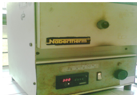
Figure 3. Furnish machine for heat treatment of NiTi T-loop spring (Material Chemistry Physic Laboratory of Bandung Institute of Technology).
