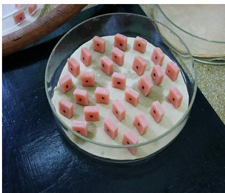
Figure 2. Testing specimens. Upper: Surface grinding on one side of acrylic plates. Lower: Marking on non-ground side of acrylic plates.
