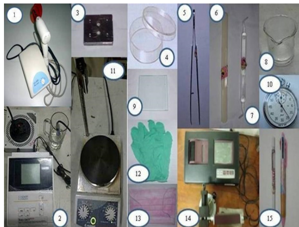
Figure 1. Research Tools: (1) Lightcuring Unit (LA 500 Blue Light, Apoza Enterprise, Taiwan), (2) pH meter (Schott Instruments), (3) Composite Resin Specimen Mold, (4) Petri Dish, (5) Tweezers, (6) Composite Spatel, (7) Plastic Instruments, (8) Measuring Cups, (9) Glass Slabs, (10) Timers, (11) Heating Stirrers (Heidolph, Germany), (12) Gloves, (13) Masks, (14) Surface Roughness Tester (Surfrest SJ-301, Mitutoyo), (15) Stationery.
