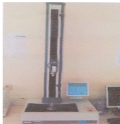
Figure 3 Pressure strength tester machine (Lrx plus llyod instrument)
