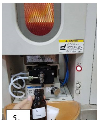
Figure 5. The solution was calculated using an Atomic Absorption Spectrophotometer
