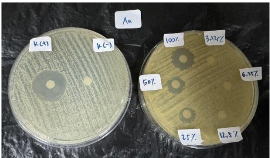
Figure 2. Photographs of petri dishes illustrate the dose-dependent antibacterial activity of green tea extract from Gunung Gambir Jember against Aggregatibacter actinomycetemcomitans . K (+), positive control; K (-), negative control; 3.125%, 6.25%, 12.5%, 25%, 50%, 100% are the green tea extract concentrations.
