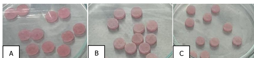
Figure 1. Disc-shaped acrylic plate sample. A. acrylic plate without a coating (negative control group). B. acrylic plate coated with a soft denture liner (positive control group). C. acrylic plate coated with a soft denture liner containing cassava starch (treatment group)
