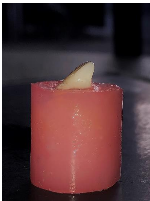
Figure 1. Specimen for the shear bond strength test.
