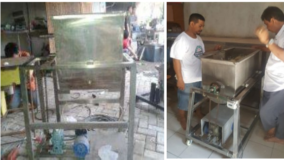
Gambar 3. Mesin pencampur ragi sistem ribbon screw
