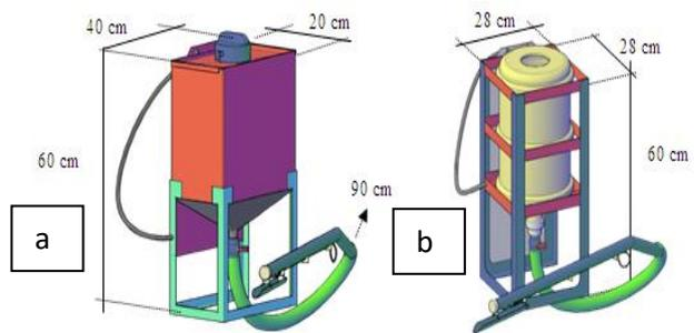
Figure 1. Design of Fertilizer Device (a) Type 1 and (b) Type 2
