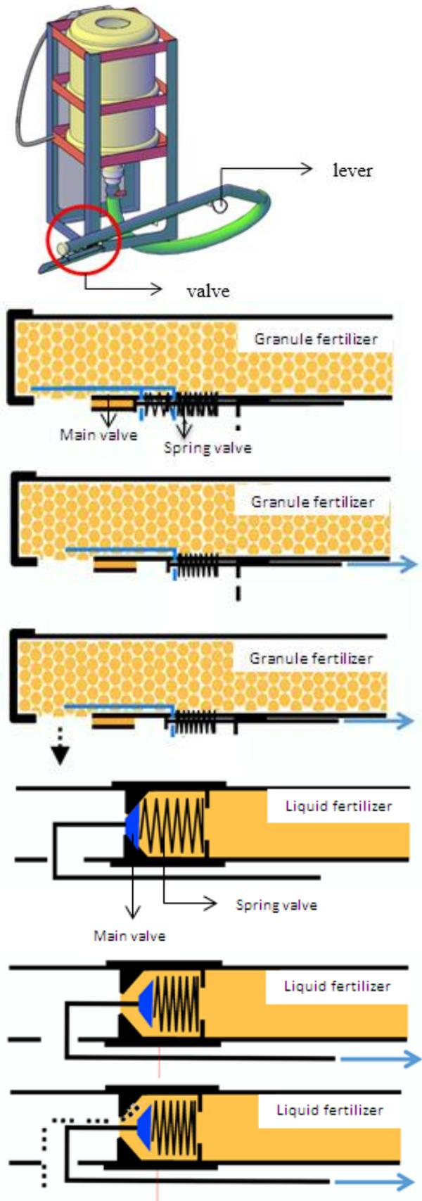
Figure 3. Work principles of a portable fertilizer device
