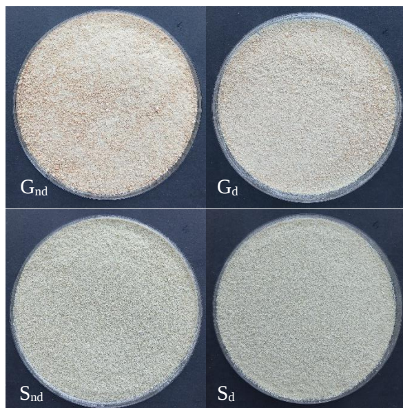
Gambar 2. Sampel Selulosa Gracilaria verrucosa non dewaxing ( G_{nd} ); Selulosa Gracilaria verrucosa dewaxed ( G_d ); Selulosa Sargassum sp non dewaxing ( S_{nd} ); dan Selulosa Sargassum sp dewaxed ( S_d )
